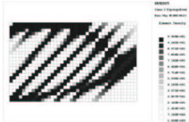
Figure 8 An 45 degree optimised cantilever beam, with constraint on volume fraction and compliance.
