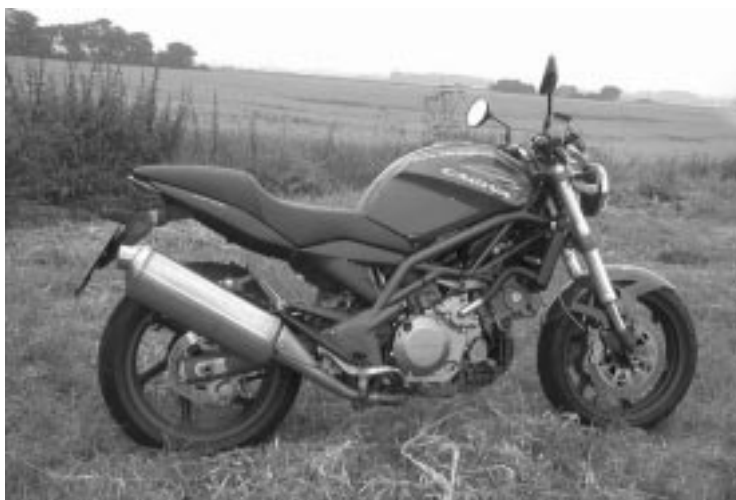
Fig. 13: Cagiva Raptor. The use of the trellis frame follows the same tendencies as in the Ducati Monster. Picture courtesy of Motorcycle Online Inc.
