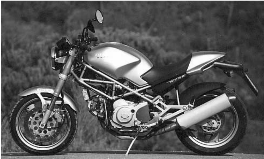
Fig. 12: Ducati Monster. The trellis frame is exposed and utilized as a shape element in the overall design. Picture courtesy of Motorcycle Online Inc.
